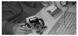
Figure 9: Transferring programs using an infrared ray
